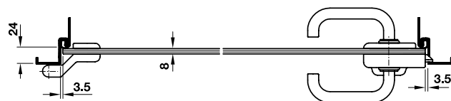
Mounting situation DIN left hand, single doors
